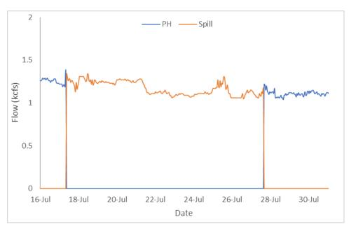
Figure 17. Hourly Flows PWR vs. Spill (Big Cliff Dam).
